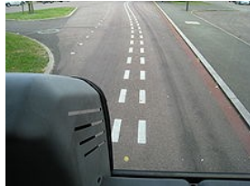
Cameras follow the lines that steer the vehicle
